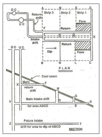
level roadways EC and ED in the seam (see plan) from point E, at right angles to the main drift YE. The roadway CED represents the main intake and conveyor level for the first pair of working faces, the loading point into tubs or mine cars being at E.
